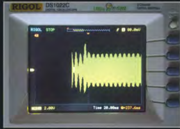
Digital storage Oscilloscope showing lamp starting conditions
